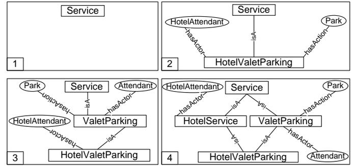
**Figure 3: Service ontology of the agent; (1) initial, (2) after adding *HotelValetParking*, (3) after adding *ValetParking*, (4) After adding *HotelService* concept.**
