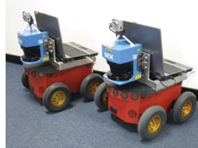
Figure 1: The P3-AT mobile robots used in this paper, equipped with onboard computers, cameras, laser and sonar range sensors.
