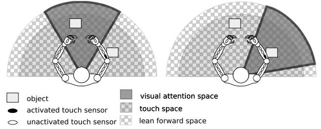
**Figure 5: The virtual human directs its sensory attention toward an object. Left: the virtual human perceives an object with the skin sensors beyond its visual attention space. The object is registered in the touch object map. Right: A motor action is selected and shifts the head and the visual attention space toward the touch-location. The object elicits a visual stimulus and is then registered to the visual object map.**
