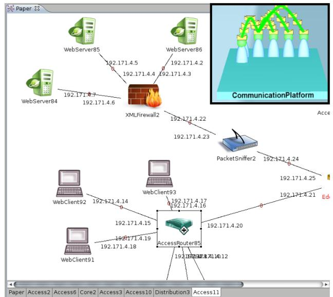
**Figure 1: GUI and Backend illustrated: The GUI enables the creation and administration of arbitrary networks and node configurations. After the setup process is finished, an agent-based simulation backend (“CommunicationPlatform”) executes the simulation and the results are stored in a database.**
