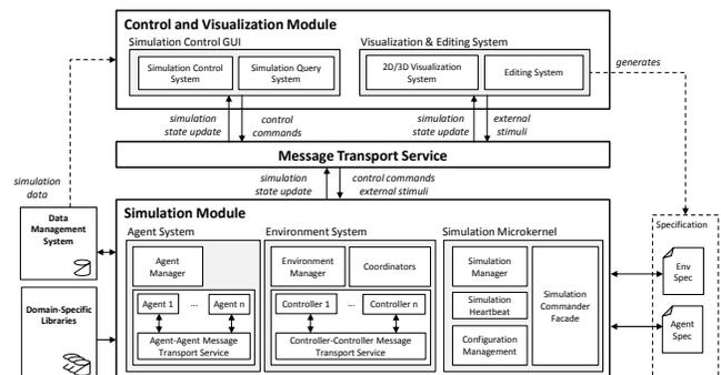
Figure 1: DIVAs framework high-level architecture
