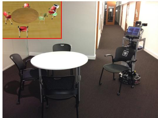
Figure 6: A snapshot from one of the real world experiments, where the task of the robot is to arrange the chairs around the round table. Visualization of the setup in simulation is provided on the top left corner of the image.
