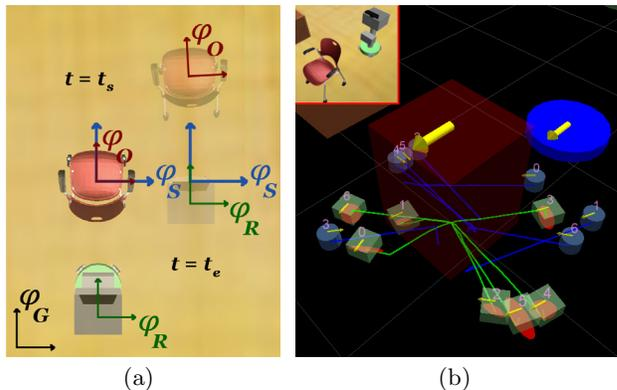
**Figure 2:** (a) Various reference frames used during sequence recording and replay depicted before ( $t = t_s$ ) and after ( $t = t_e$ ) a push. (b) Visualization that corresponds to the scene shown in the upper left corner of the image (best viewed in color).
