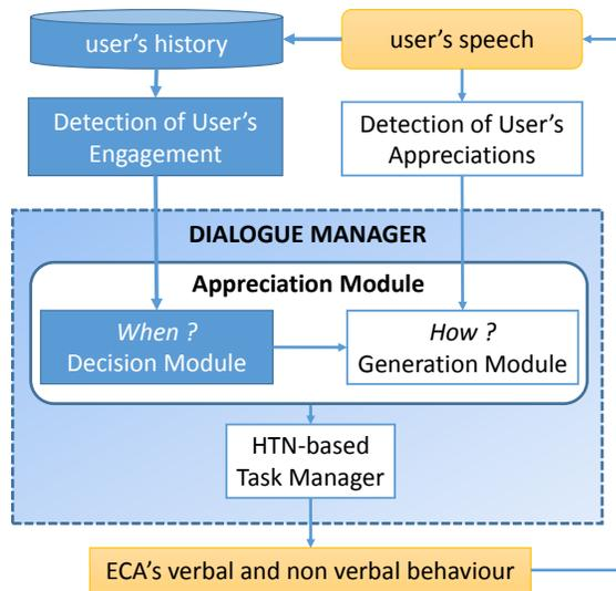
**Figure 1: General architecture of the appreciation module**
