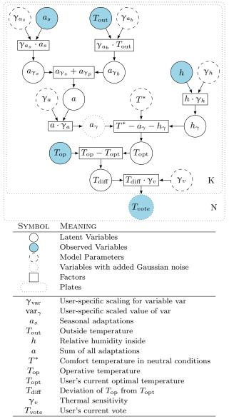
Figure 1: The personalised thermal comfort model as a Bayesian network (with nomenclature)
