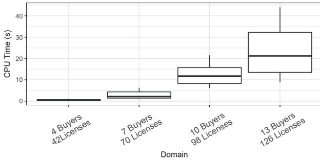
**Figure 2: Run-time results for finding the efficient allocation using our MIP formulation for differently-sized problems. The box plot provides the first, second and third quartiles; the whiskers are at the 10th and 90th percentile.**
