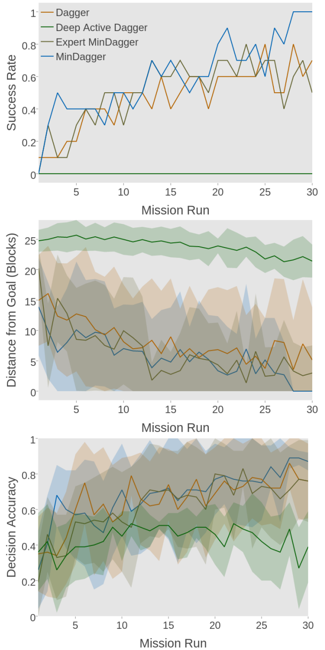
Figure 6: The average success rate (top), distance the agent is from the goal at the end of each mission (middle), and the average decision accuracy (bottom) compared to the training policy for each run through the random set of mazes.
