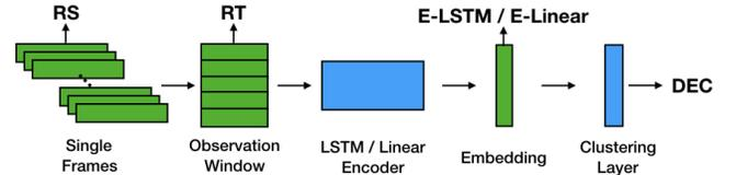
**Figure 1: Visualization of our entire role discovery pipeline with our different baselines. RS: Raw Single frame data. RT: Raw Temporal data. E-LSTM/E-Linear: Embeddings +  $k$ -means. DEC: Full DEC network output.**
