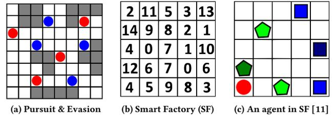
**Figure 2: (a) Pursuit & Evasion ( $N = 4$ )** with pursuers (red circles) and evaders (blue circles). **(b) Machine grid of the Smart Factory (SF)** with the numbers denoting the machine type. **(c) An agent  $i$  (red circle) with  $tasks_i = \{\{9, 12\}, \{3, 10\}\}$  in the SF of Fig. 2b.** It should get to the green pentagonal machines first before going to the blue rectangular machines [11].
