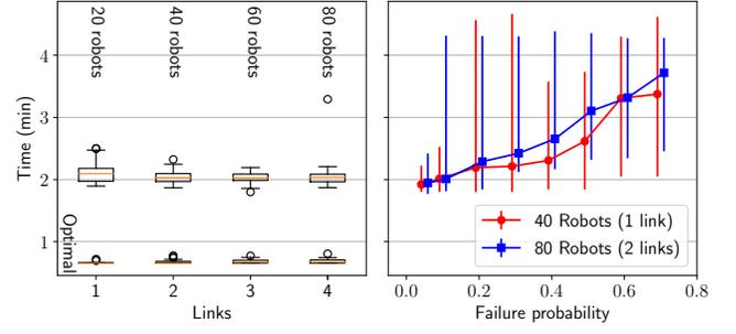
**Figure 2: Time to build chains with 20, 40, 60 and 80 robots without failures (left); time to build chains with 40 and 80 robots and with varying failure probability (right).**
