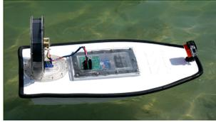
**Figure 2: Platypus<sup>2</sup> Lutra boat used in the context of the INT-CATCH project, about 1 m long and 0.5 m wide.**
