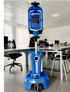
Figure 7: Giraff-X socially assistive robot, developed for the MoveCare project [28]
