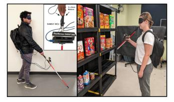
Figure 1: The system is comprised of a robotic cane equipped with RealSense D455 and T265 cameras. The system is powered through a laptop in a backpack. *Left*: Utilizing haptic feedback for navigation guidance. *Right*: Utilizing audio cues for manipulation guidance.
