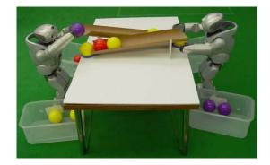
Figure 1: QRIO robots performing ball sorting task.
