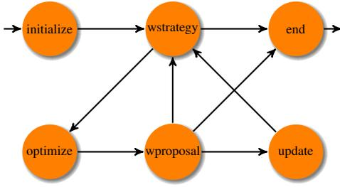
**Figure 1: Finite state machine for distributed negotiation**
