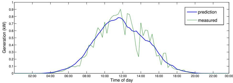
Figure 9: Power prediction of one PV panel
