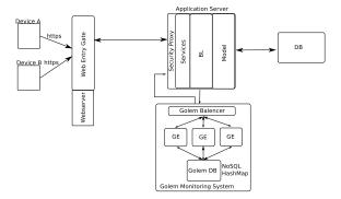
Figure 1: Overall architecture of the GDMMS
