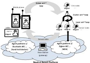
Figure 1: The self-StarMAS global architecture
