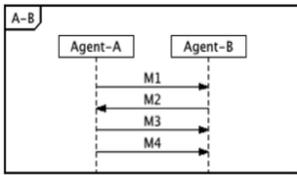
Figure 1: AUML Protocol With No Constructs
