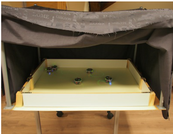
Figure 2: Darkroom with glow-in-the-dark floor. The e-puck robots circle around and emit UV light to the floor.
