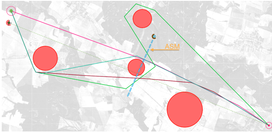
Figure 2: Screenshot of the UAV control display proposing several alternative trajectories. Live demo can be found at: http://agents.cz/arethus/UAV-HMI.avi
