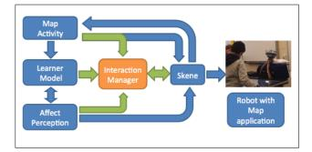
Figure 2: The Emote Architecture configuration for empathic interaction using the touch table map reading application and the physical robot
