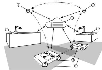
**Figure 1: Overview of the considered setup with (1) a holonic (multi-agent) coordination system, (2) automated guided vehicles, (3) work stations and (4) a localisation system composed of different camera modules with their corresponding field-of-view depicted by (5). Arrows indicate the communication flow between the different agents.**
