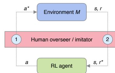
**Figure 1: Oversight in HIRL.** At (1) human overseer (or Blocker imitating human) can block unsafe actions  $a$  replacing them with safe actions  $a^*$ . At (2) overseer delivers a negative reward  $r^*$  for unsafe actions.
