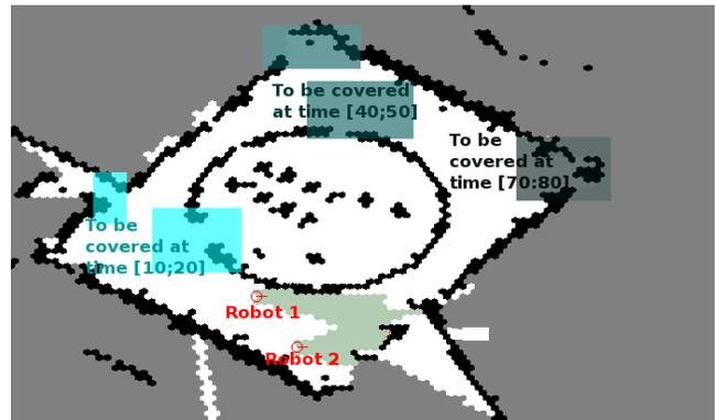
**Figure 1: A rescue-support example: the robot team must cover the various Areas of Interest (AoI) at given timesteps. For best covering all the AoI, robots should tightly coordinate for positioning themselves in order to best share the AoI at time [10,20]. Then, robots should split, one for being in time for covering the top [40-50] AoI and the other for covering the [70-80] AoI.**
