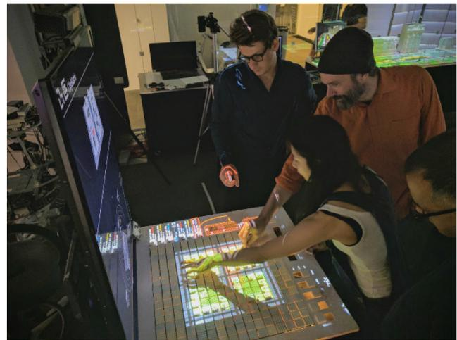
Figure 1: CityMatrix – an urban decision support system with a tangible user interface, real-time feedback of multiple urban simulations, and optimized suggestions
