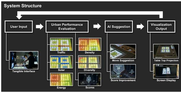
Figure 2: Software structure of CityMatrix.
