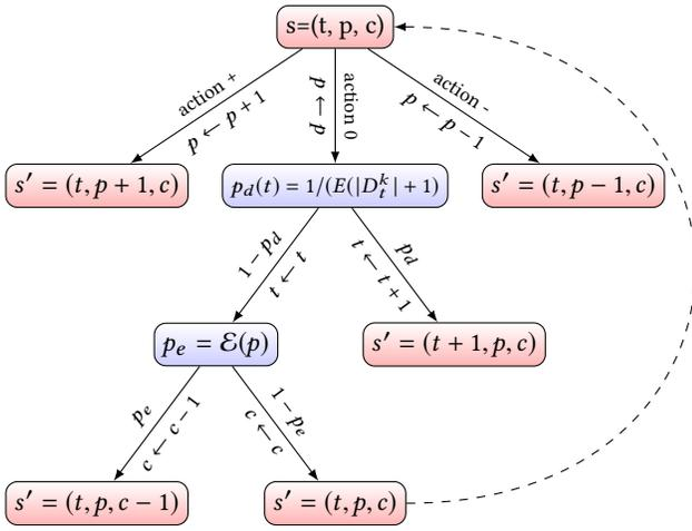
**Figure 2: The structure of the transition function  $P$ .** Given state  $s$ , the probability of getting to the next state  $s'$  is given by multiplying the probabilities along edges. States are the decision nodes (in red), chance states are in blue and contain the definition of the probability used on the edge.
