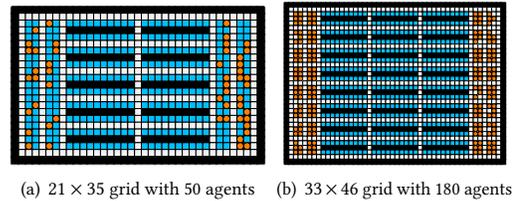
**Figure 4: Two 4-neighbor grids that represent simulated warehouses. Black cells are blocked, blue cells are task endpoints (pickup locations and/or delivery locations of tasks), and orange circles are non-task endpoints (both start and parking locations of agents).**
