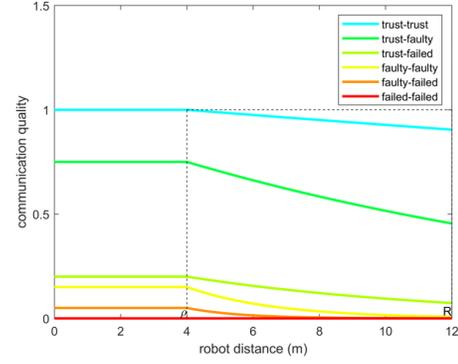
**Figure 3: Illustration of the Trust-aware communication quality assessment. Information shared by trusted robots is encouraged with higher upper limits, while untrusted information is discouraged with lower upper limits.**
