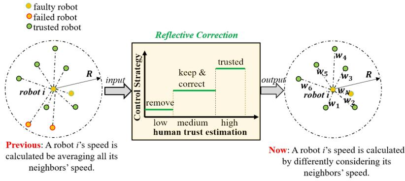
Figure 2: Illustration of change in speed calculation in the Trust-Aware Behavior Reflection for Swarm Self-Healing.
