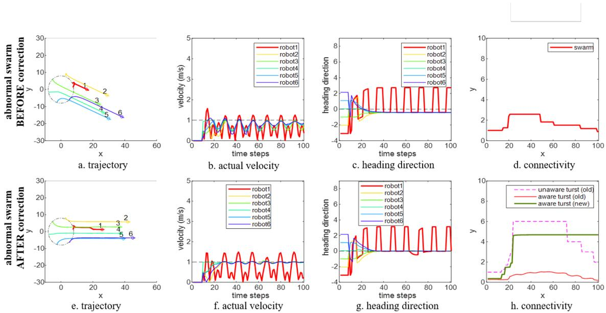
Figure 6: System response given by untrusted behaviors caused by system uncertainty (faulty sensor).
