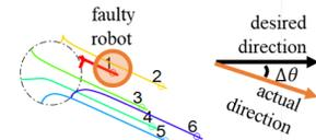
**Figure 1: Undesired swarm flocking caused by faulty robots sharing incorrect information with their neighbors.**
