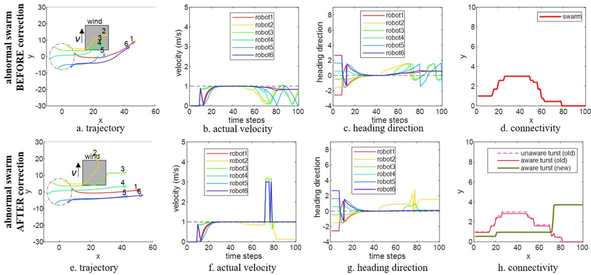
Figure 7: System response given by untrusted flocking caused by a wind disturbance.
