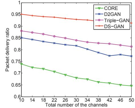
Figure 7: Comparisons on the packet delivery ratio when fixing  $M$  and varying  $N$
