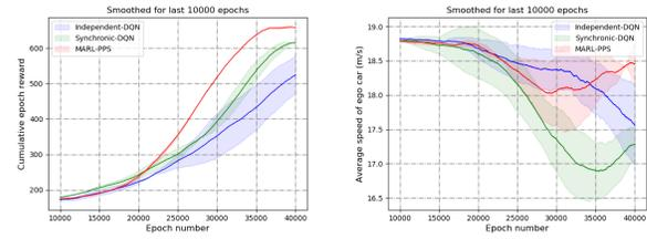
**Figure 3: Training curves for baselines and the proposed algorithm. The left plot shows the mean epoch rewards for different methods. The right plot is for the average speed of the agents.**
