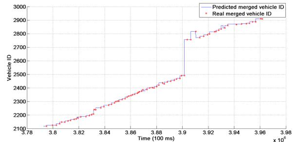
**Figure 3: Prediction output of the proposed model: the curve is increasing because the ID of the vehicle crossing the merging point is unique and increases over time.**
