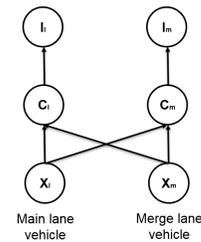
**Figure 1: DBN used for highway on-ramp merge situation.**
