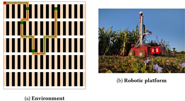
Figure 1: (a) The robot (red cell) determines the  $p$  most informative samples (here  $p = 4$ ) in the field which are shown in green and finds the most informative path (green arrows). (b) Robotic platform used for collecting data.
