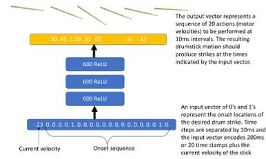
**Figure 2: The network is trained to produce a sequence of actions controlling the drumstick’s trajectory. The resulting trajectory should produce a rhythm that is identical to the sequence provided by the input vector.**
