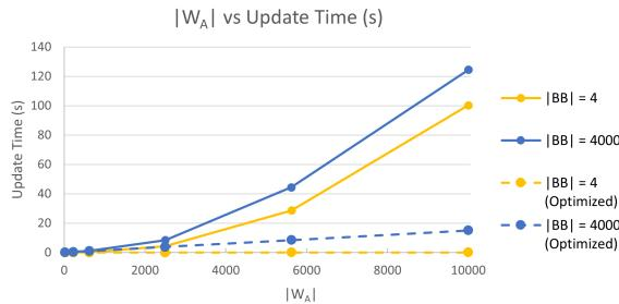
**Figure 8:**  $|W_A|$  vs. Model Update Time (s), where the solid and dashed lines represent the original and optimized implementation, and the yellow and blue lines represent updates where  $|BB| = 4$  and  $|BB| = 4000$ , respectively.
